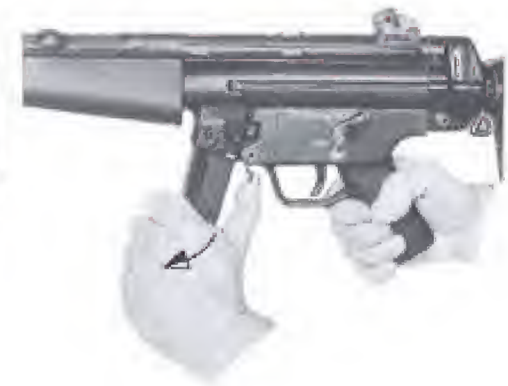
Fig. 25 Removing the magazine
